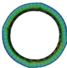
Cutting Balloon Maximum stress 3.109 MPa
