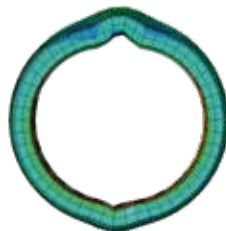
Dual Wire Scoring Balloon Maximum stress 2.036 MPa
