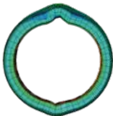
Dual Wire Scoring Balloon Maximum stress 2.036 MPa
